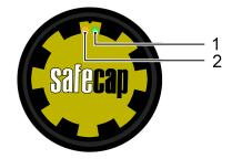
Green LED (1) and yellow LED (2) are lit up. Process on the machine not triggered.
